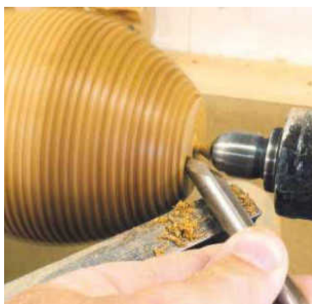
STEP 27. A small tool and small cuts are the order of the day here. What you don't want to do at this stage is to experience a dig in. There will be short-grain in the foot so don't go too thin. The last bit can easily be finished by hand
